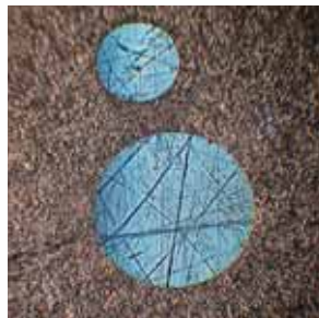
Holes cut by laser in tungsten (0.5 and 0.3 mm diameters)
