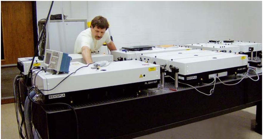
Nearly Fourier transform limited 30 ps tunable pulses for advanced spectroscopy.
